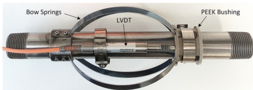
Figure 2. Picture of the Phase 1 LVDT device constructed to measure borehole closure
