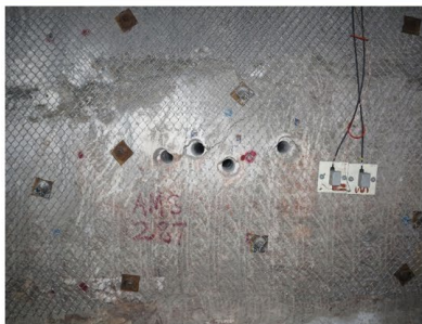
The face of the wall on which the horizontal boreholes are located for shakedown experimentation.
