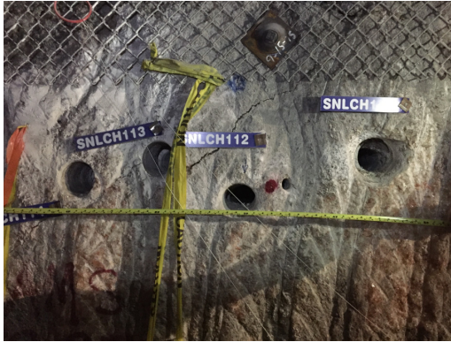
Figure 2.2: Configuration of existing boreholes used in phase 1 testing installation of an infrared heater in the WIPP underground.
