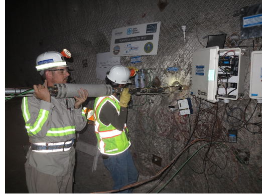
Figure 2.2: Configuration of existing boreholes used in phase 1 testing installation of an infrared heater in the WIPP underground.
