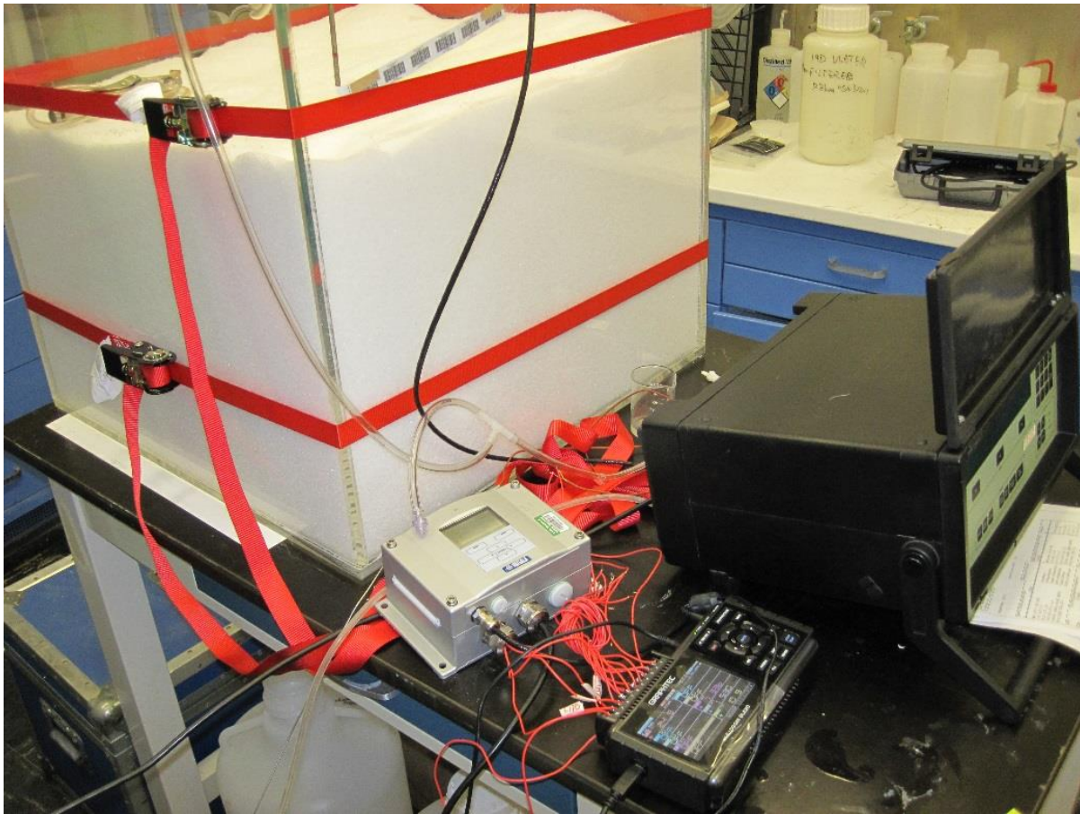
Figure 4. Salt box, data loggers, and multi-gas monitor.
