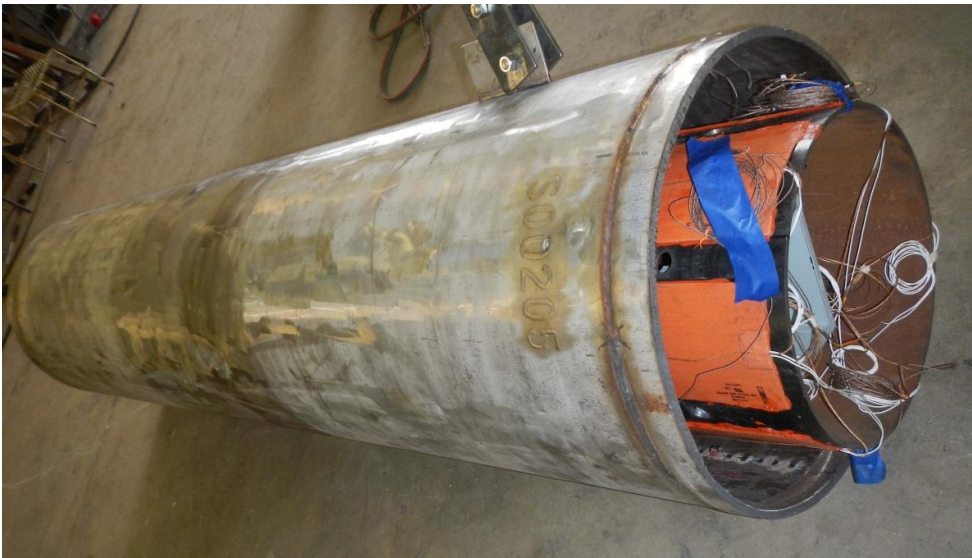
Figure 18. Heating harness inserted into canister.
