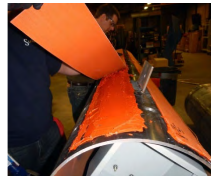
Figure 4: Adhering strip heaters to 16" pipe
