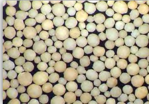
Figure 8: Cerabeads #850 sieve size (.010 mm)
