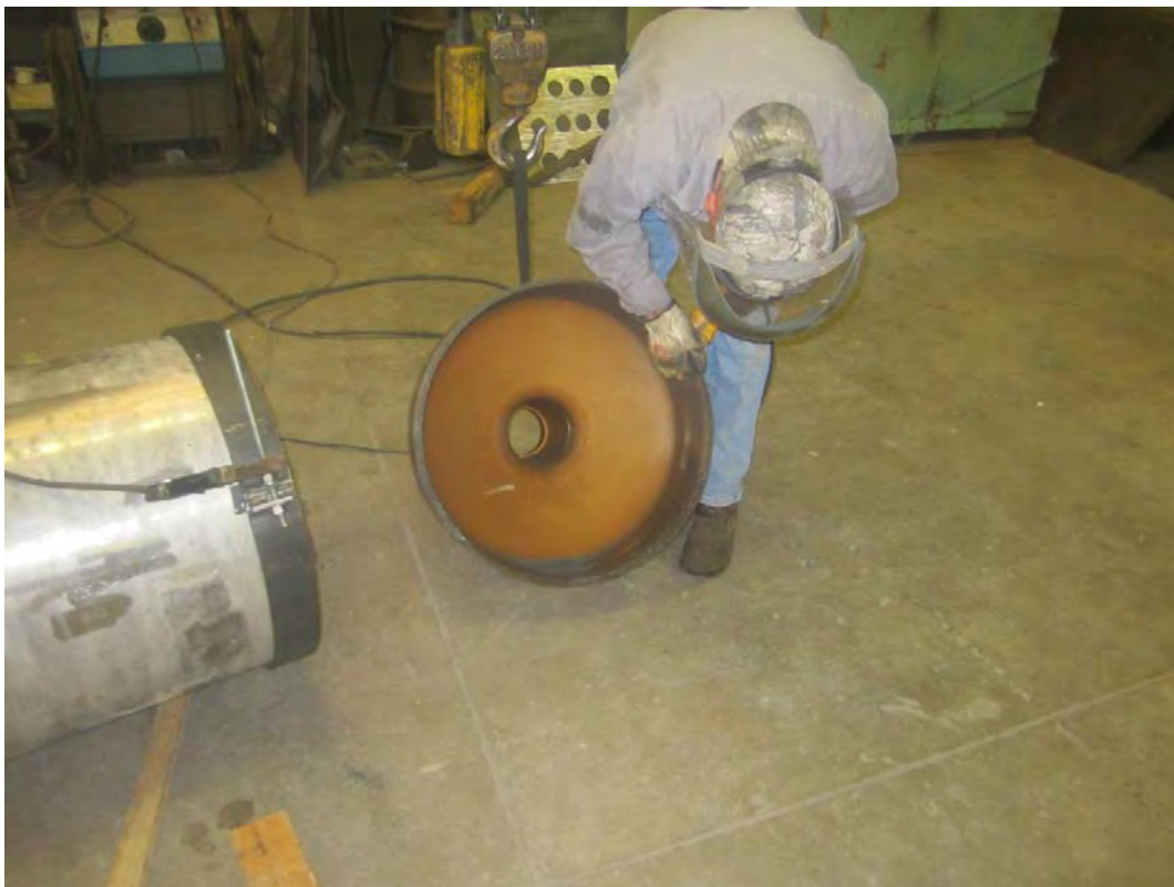
Machinist Beveling Canister Cap with Grinder
