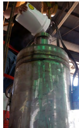
Figure 5: Filling with Cerabeads
