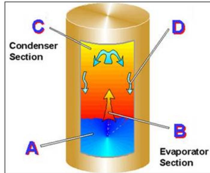
Heat pipes lead to isothermal regions where phase change is absorbing energy
