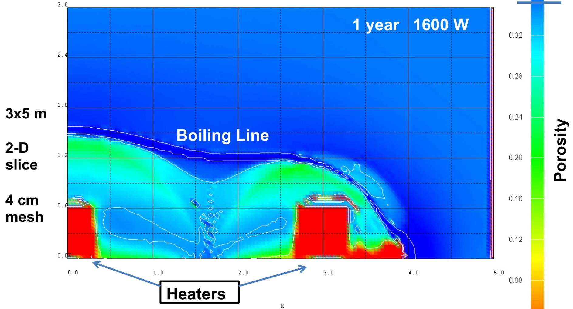
**Boiling near the heaters causes salt to precipitate leading to porosity reduction. Vapor condenses across the boiling line leading to dissolution and increased porosity**
