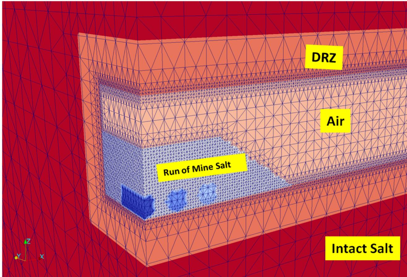
*2 Reflection boundaries are used to reduce mesh size (1/4 space)*
