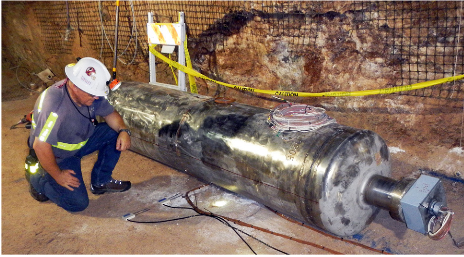
Fig. 3. External view of the complete canister assembly, placed on the drift floor of the Waste Isolation Pilot Plant prior to the addition of the run-of-mine salt pile.
