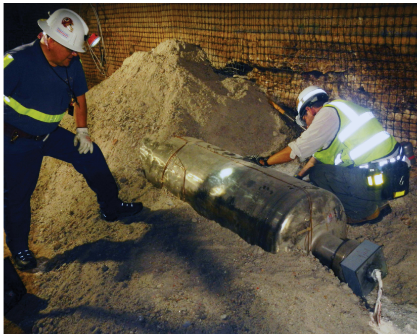
Figure 7. Heater buried under a pile of WIPP Run of Mine salt [33].
