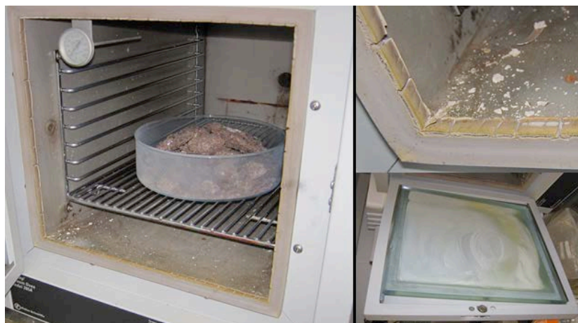
Figure 2. Oven Corrosion after Heating WIPP salt from Clay Seam F.
