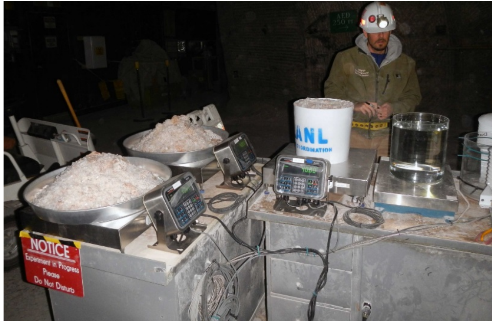
Figure 2: Salt pan experiment in WIPP salt gallery. Pans with salt piles are on left.
